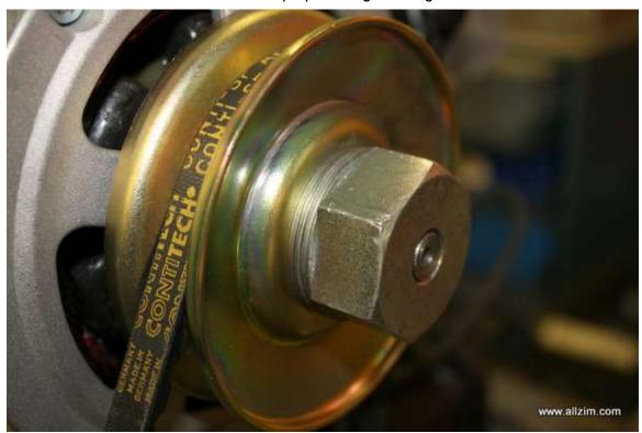
Now look from the side of the engine just to make sure the alternator pulley and the crank pulley are in line and the belt is running true. If the pulleys seem to drag on something look at the little tab on the top section of the alternator which is used to
