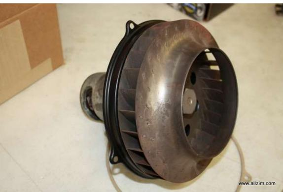
Once the assembly is out and on the bench you must remove the large nut that retains the fan to the back of the generator. There are two ways this can be done. If you have
