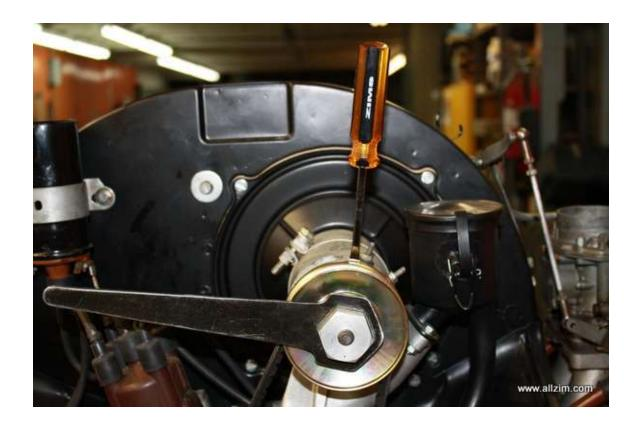
Remove the nut, belt, all of the pulleys, and shims. For now leave the pulley hub and the woodruff key mounted on the generator as you might need it to loosen the fan nut later. You **will** be re-using these parts unless they are damaged. If so, call us and we can supply you new pulleys, hubs or nuts. Make sure you have enough shims to put it all back together. It is wise to keep spares to put in your emergency tool kit.
