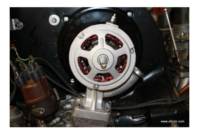
Pre-form (bend) the new supplied T-bolt style alternator strap around the bottom of the alternator stand and up and around the alternator in a position that fits nicely and arrange the end where the bolt goes through so it can be accessed easily to tighten it. This is putting the clamp on where the nut on the bolt faces towards the left of the alternator and the t-bolt running horizontal on the bottom under the alternator. Do not tighten yet.
