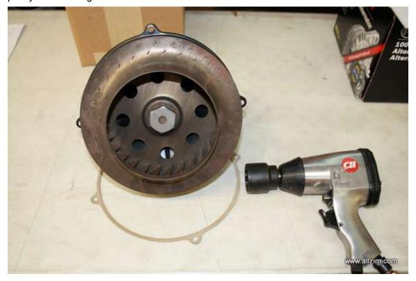
Loosen the 36mm large nut with a socket and breaker bar. Once the nut is off the fan, remove the spacer washer and fan and shims if any are there. You will be reusing the thick washer and the nut back if undamaged. We can supply you new parts if any of these are damaged. If your fan has a small disc or plate covering the center holes on the fan, discard it. It cools better if these holes are open.
