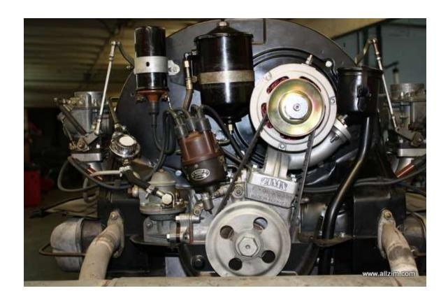
Remove the large 36mm (1&7/16") nut on generator holding the pulleys and shims together. It is important to use the proper tools to do this and not damage the hardware. Use the supplied special ZIMS square shafted screwdriver / pulley holder tool to hold the pulley in the notched area against the generator housing to lock the shaft and loosen the nut.
